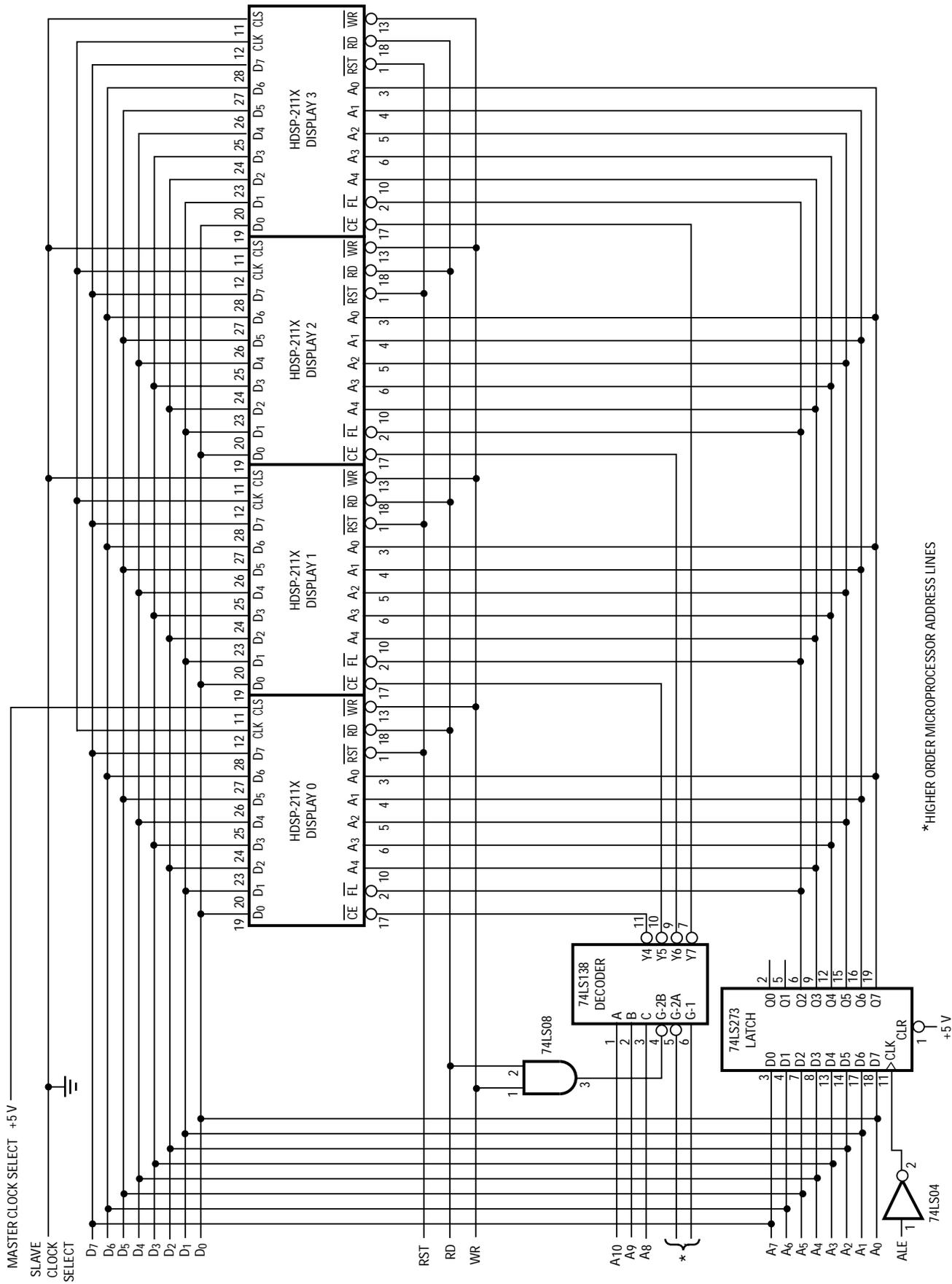
Figure 15. Character interface to 8085 Microprocessor
