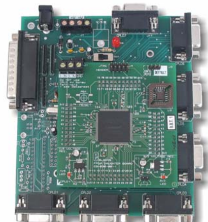
The FPGA board fits on top of the CPLD programming board – like this:
